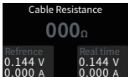
Measure the internal resistance of the cable using the pressure difference method, which requires the use of a constant current load.
